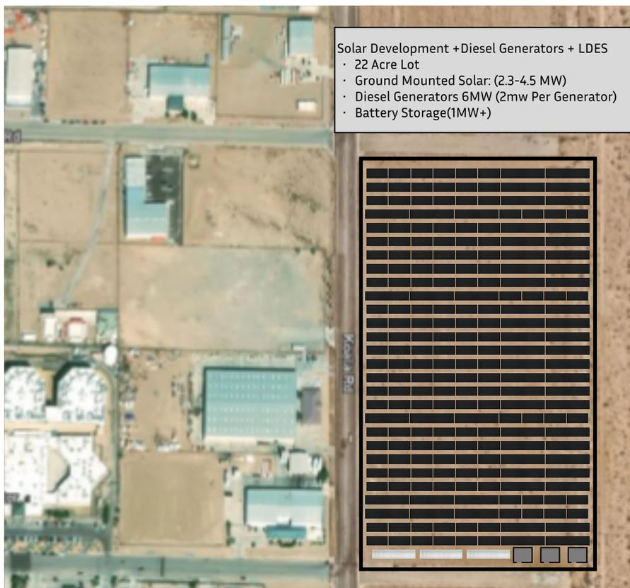
\*\*\*Refer to system spec for solar, diesel and battery estimates
